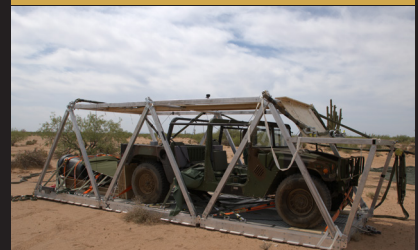
Fig 3: Air bag landing, de-rig <10 mins
