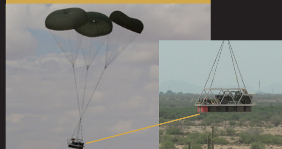
Fig 5: Safely delivered under G11 cargo parachutes, with airbag landing
